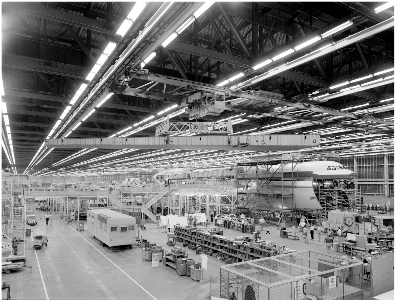
Right-hand outer wing of C-5A being lifted to wing dock by an aerial crane, November 1967.
