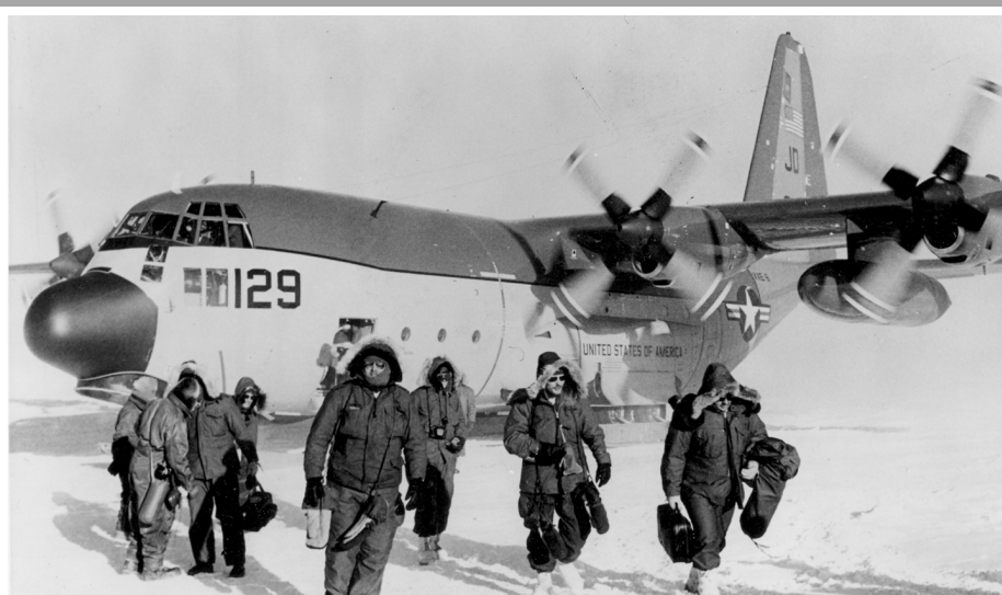
The Navy version of the C-130E, the LC-130R, equipped with Teflon-coated skis, was delivered to the National Science Foundation and U. S. Navy's VXE-6 squadron in Antarctica in 1974. Note the underwing fuel tanks.
