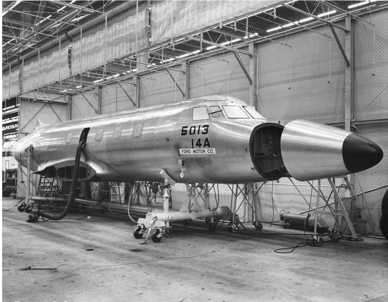
Ford Motor Company JetStar in production, ca. 1960. Many JetStars were sold in advance and the name of the customer was placed on the side on the assembly line. A sign on one of these special orders reminded workers that future orders from that company depended on the quality of their work.
