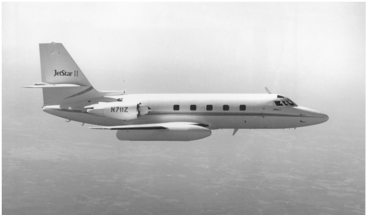
The JetStar II was an improved version of the corporate jet produced by the Marietta plant in the 1950s. This is one of 40 that were made, ca. 1977.
