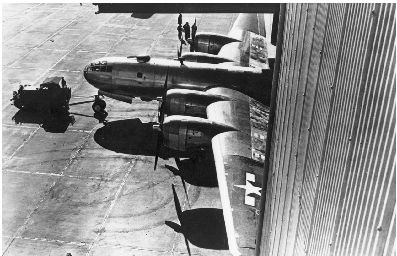
Roll out of the first B-29, November 1943. With jigs and tooling still being developed, the first few aircraft were constructed largely by hand.
