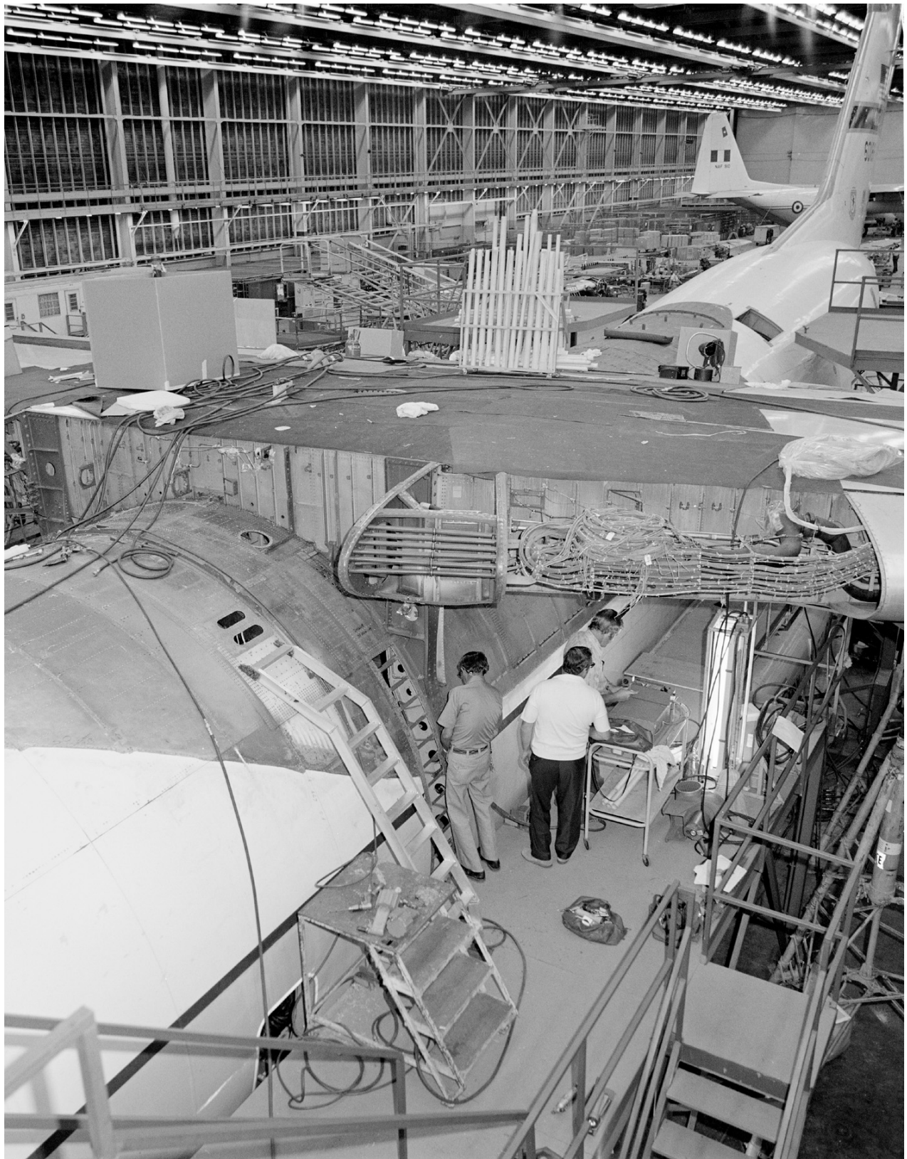
Extra fuselage sections and other modifications are given to a C-141A Starlifter as part of the "stretch" program to increase its cargo capacity, July 1976. The 270 modified planes were re-designated C-141B.
